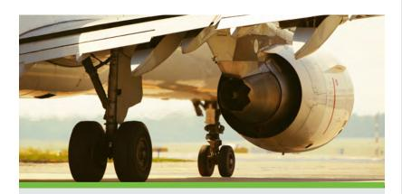
Aerospace processes commonly use fluorescent magnetic particles and NDT-approved carrier oils for safety critical ferrous parts including steel alloy landing gear.
